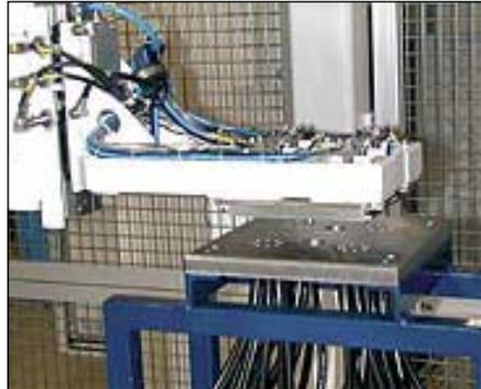
The Hekuma handling system for Stamm's tiny ballpoint pen nozzles sorts the parts by cavity. The tubes below the receiving plate carry the parts by vacuum pressure to individual containers that can be checked while the system is running.
