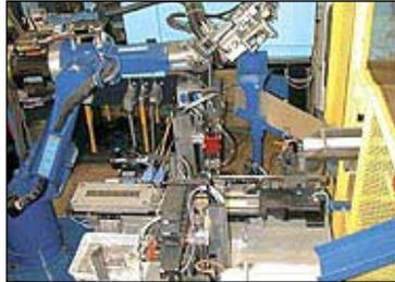
Stamm AG see robots as necessary for micro-part quality maintenance. With this Reis six-axis system, it has combined pick and place with assembly and sorting functions for a complex part with inserts.
