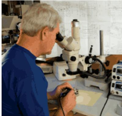
Mold assembly is done under a microscope.
