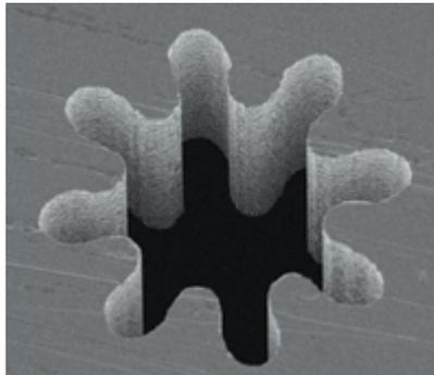
The gear mold insert was made via EDM using .03-mm wire.
