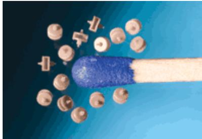
Stamm's watch rotor weighs .001g. The eight teeth of the gear on the axle have a draw of .04 mm.
