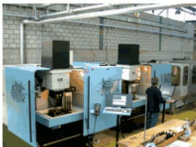
To make the gear inserts, Stamm modified one of its existing Agie wire-cut machines to use .03-mm wire that it sourced from Japan. Wire guidance had to be ultraprecise to keep from breaking that skinny wire. Stamm says it “only” took six months until the teeth were perfect.
